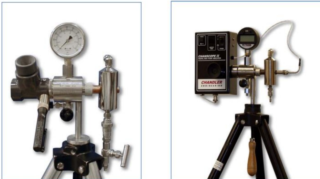
Figure 27. Two chilled mirrors in manual configuration. Image from Potter (2011) [97].
