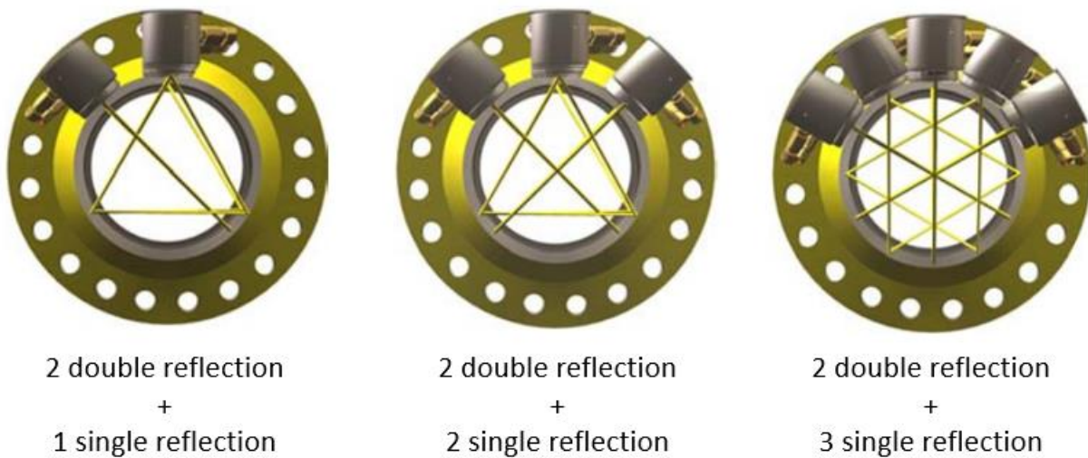
Figure 12. Principal acoustic paths configuration. Image elaborated from Dell'Isola et al. (1997) [33].
